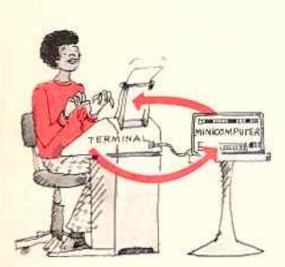
As the drawing at the left suggests, there are at least two parts to a minicomputer "system" (that's what "system" means — something with several parts). There is the box labeled MINI-COMPUTER and there is also an object called a TERMINAL. The terminal looks something like a typewriter. It is the means by which you and the computer will "talk" or communicate with each other.
